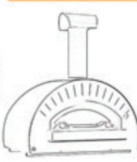
Portable Grill Ovens: Small and convenient - but with no thermal mass, heat concentrates around the flame and you lose the even, all-over heat. Risk of scorching and undercooking.
